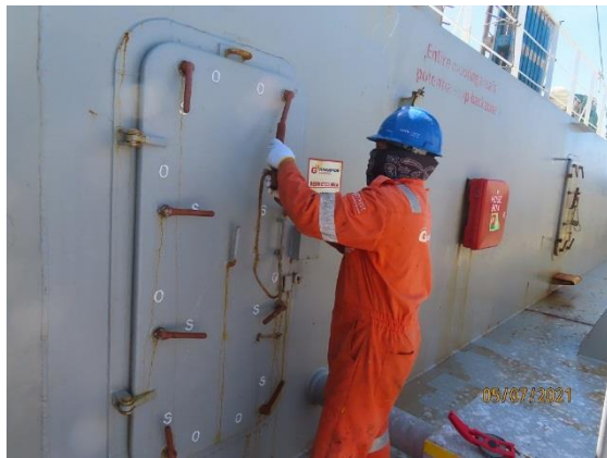
Securing All Watertight Doors
