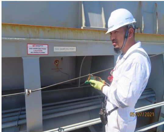
CNO continuously monitoring of Tank Atmosphere
