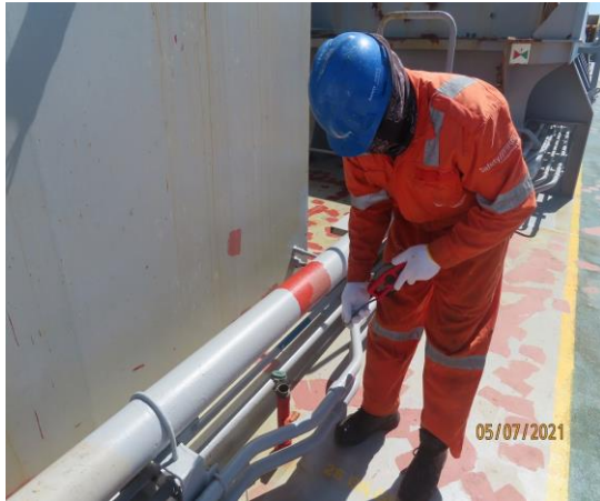
Ballast & Bilges sounding in WBT No. 2 & CHold No. 2 Bilges
